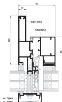
mullion with window, section view MB-SR50N IW – standard variant
